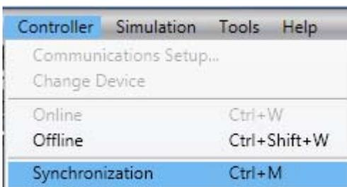
10 The Synchronization Dialog Box is displayed. Confirm that the data to transfer (NJ501 in the right dialog) is selected. Then, click the **Transfer To Controller** Button.
